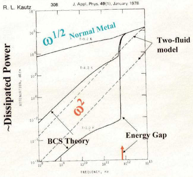
FIG. 2. Attenuation as a function of frequency for the example stripline. Solid lines are for the Mattis-Bardeen theory and dashed lines for the two-fluid model. For  $T>9.2~{\rm K}$  both conductors are normal and the two theories give the same result.
